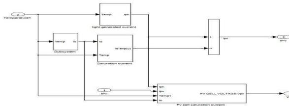
Fig 4. Simulink Model For Solar PV Cell
