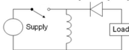
Figure 1: The basic schematic of an inverting buck–boost converter.
