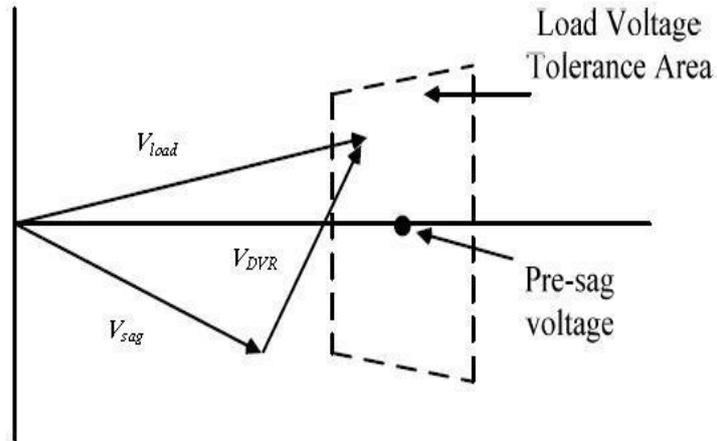
Fig. 5. Voltage tolerance method with minimum energy injection
