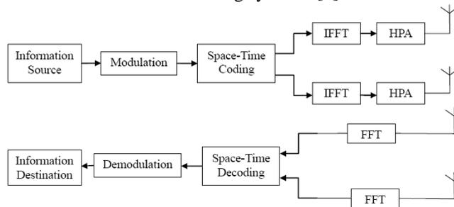
Figure 1. Basic Structure of MIMO OFDM System
