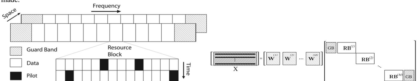
Figure 2. Data structure of an OFDM block for a MIMO-OFDM/A downlink
