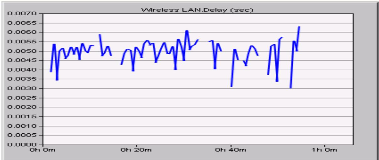
**Figure Variation of Delay for DSR Protocol**
