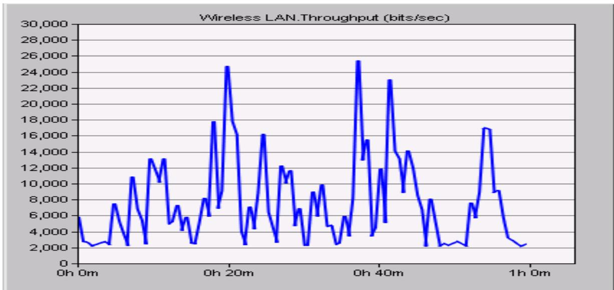
**Fig: throughput for TORA Protocol.**
