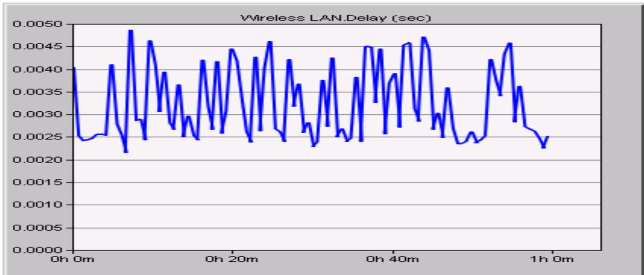
**Figure Variation of Delay for TORA Protocol**
