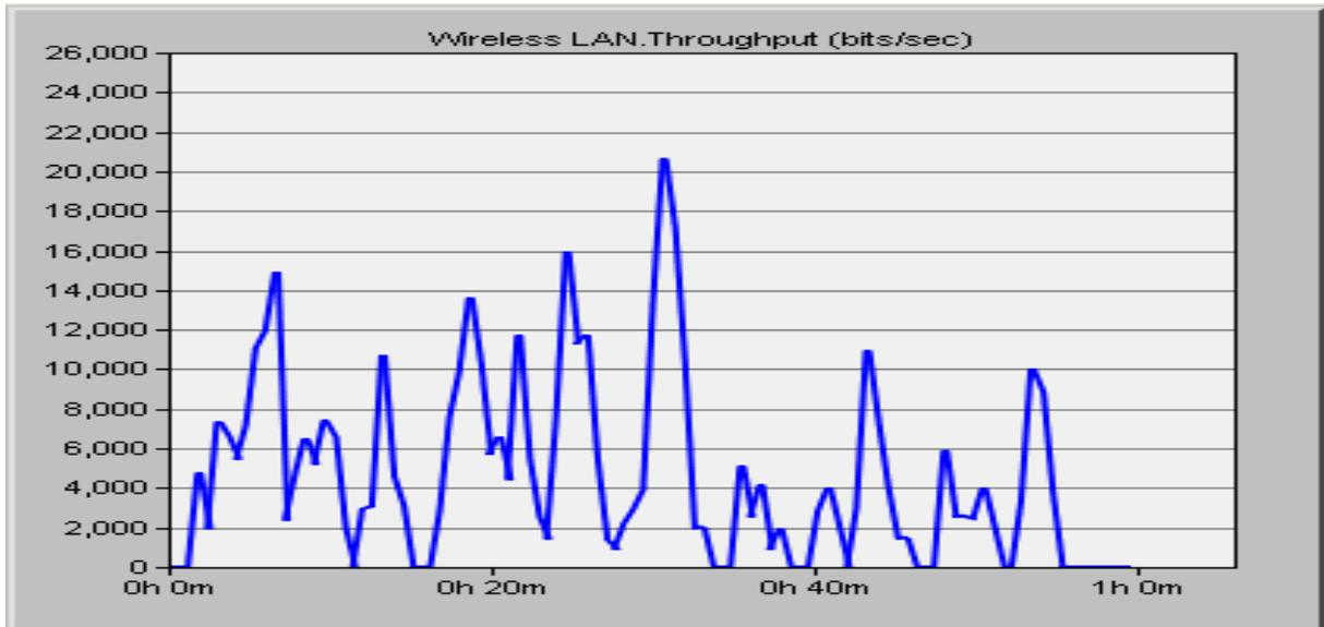
**Fig: throughput for DSR Protocol in MANET network**
