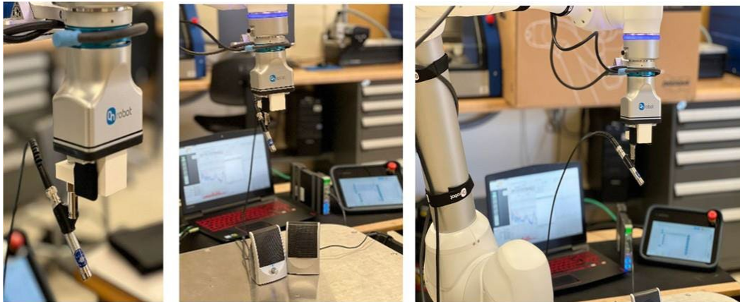
Figure 6. Doosan Robot Equipped with a Microphone that follows a Well-Defined Trajectory.
