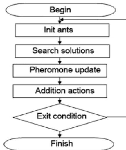
Figure 3: Ant Colony optimization flow diagram
