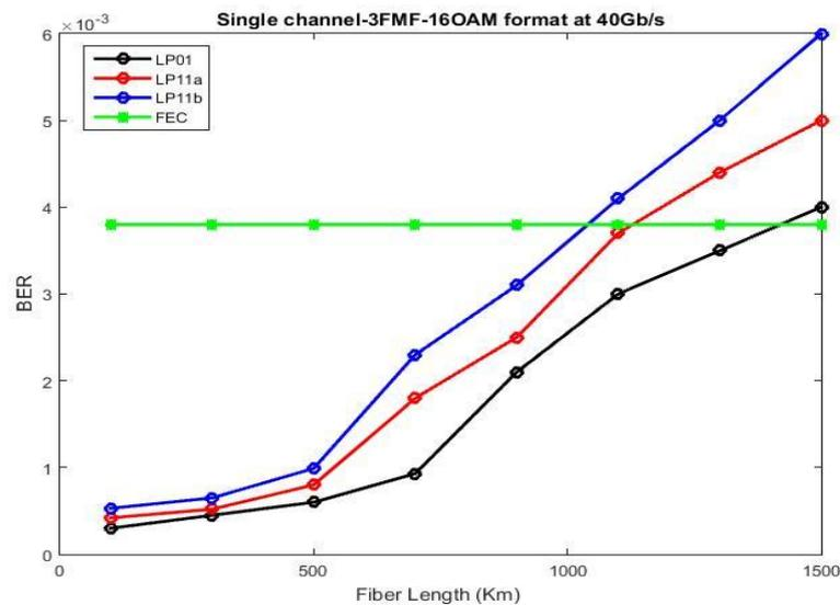
**Figure(11):** Diagram of LP modes specifying BER versus length for single channel 3-modes SDM/PDM-16QAM system.
