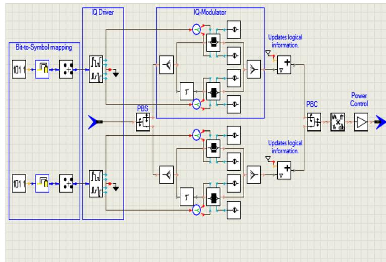
Figure (4): The block diagram of optical channel
