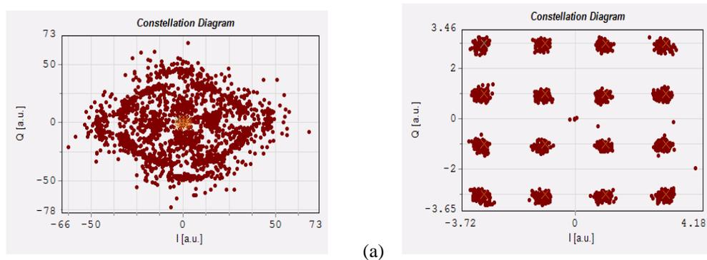
**Figure (9):** Received constellation diagram of channel 1X in LP01 mode (a) without using TDE MIMO equalizer, (b) using TDE MIMO
