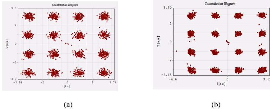
**Figure (8):** Received constellation diagram of channel 1X in LP01 mode a. Without using gray mapping ,b. Using gray mapping
