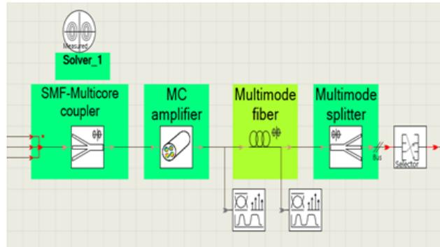
Figure (3): Block diagram of Tx-DP-modulation module
