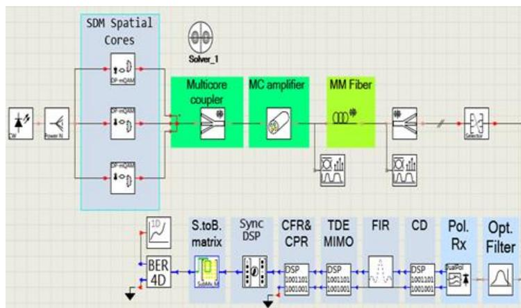
Figure (1): Single channel PDM-SDM System
