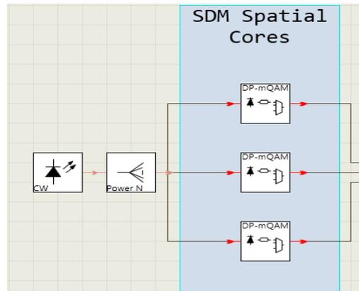
**Figure (2):** Transmitter section of 3-modes SDM System
