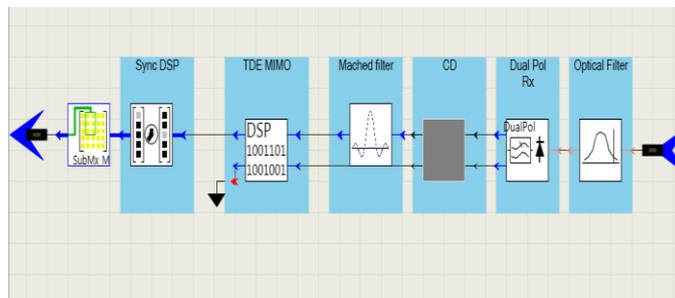
**Figure (6):** Block diagram of single channel receiver section
