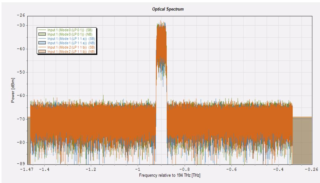
**Figure (7):** The spectrum of Optical OSA for single channel 3-modes SDM/PDM 16QAM system
