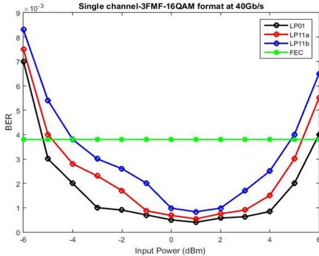
**Figure(10):** Input power versus BER for single channel 3modes SDM/PDM-16QAM system
