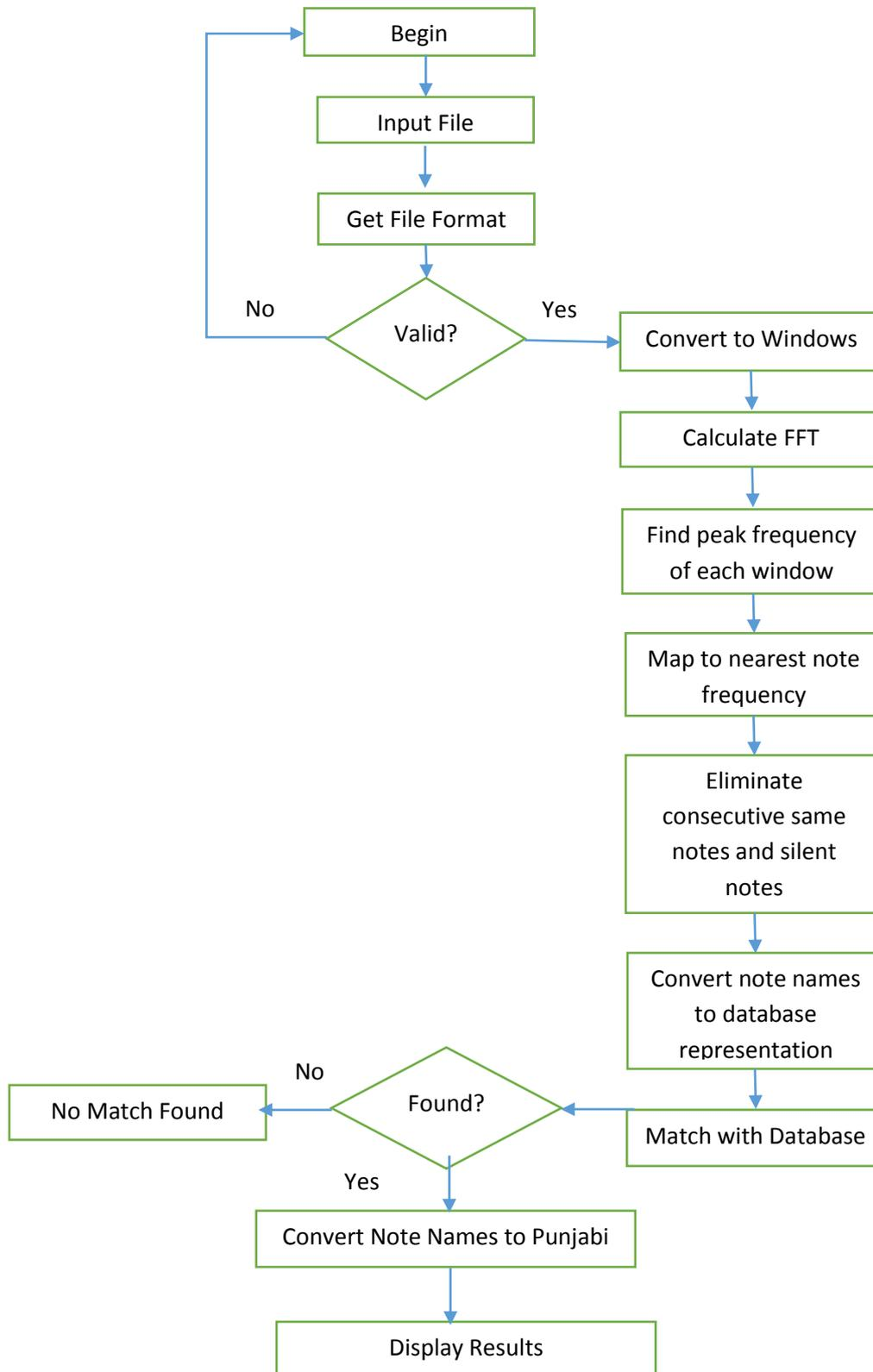
Fig. 2: The flowchart of the main working algorithm of the source code.
