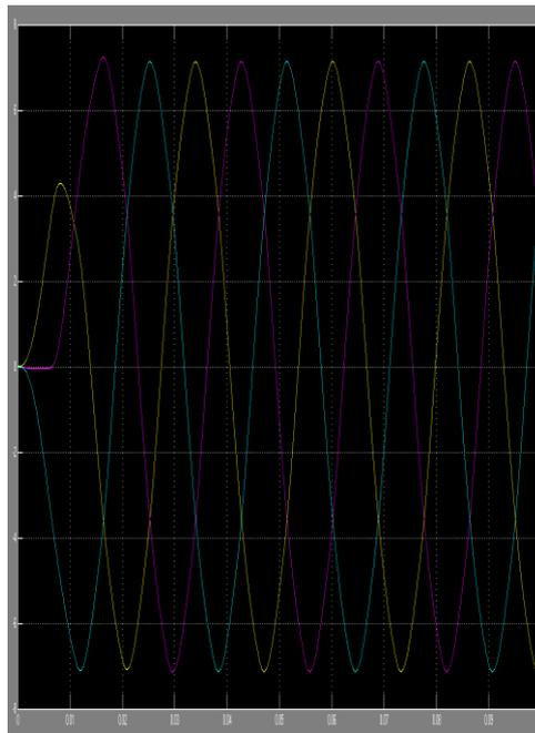
Fig6: - Current wave form after the second order Filter
