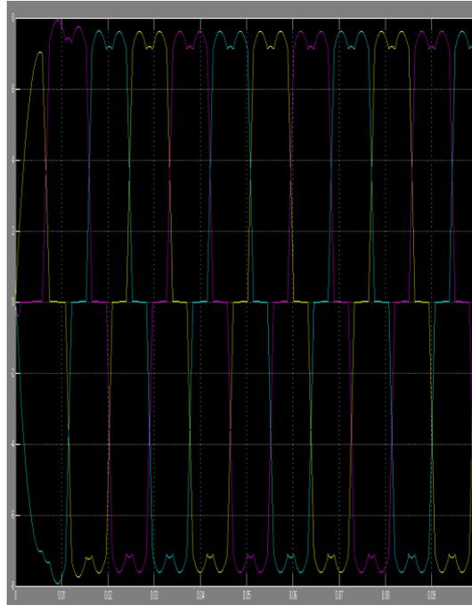
Fig5: - Current wave form before the second order filter
