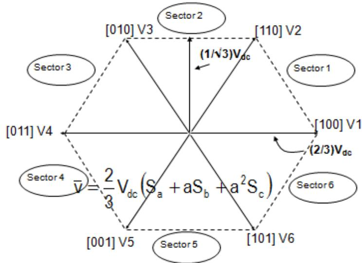
Fig1:- Space vector pulse width modulation
