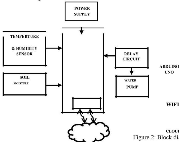
Figure 2: Block diagram
