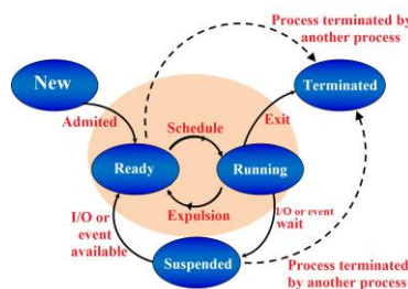
Figure 1. State diagram of process scheduling
