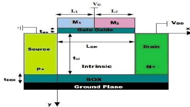
**Fig.2.** Schematic diagram of a DMG TFET
