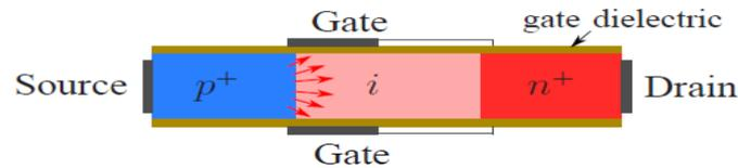
Fig.1. Double gate TFET with full (solid) and short (dashed) gate
