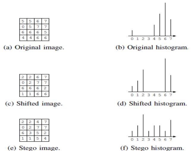
Fig. 3 Example of histogram modification
