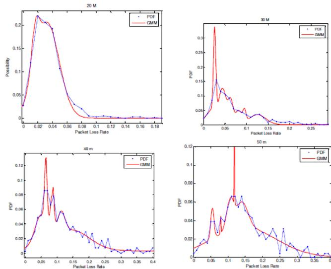
Figure2 GMM and PDF with distance range 10-20m,20-30m,30-40m,40-50 m
