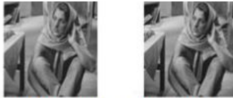
Figure 11: The original image (left) and the watermarked image with 16298 byte hidden data and 34.04 db PSNR (Right).
