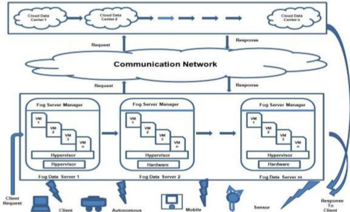
Figure 2: Fog- Cloud Three Layer Architecture [3]
