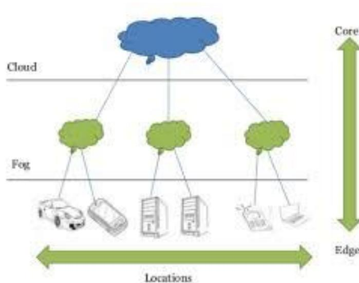
Figure 1: Fog Computing Architecture [1]
