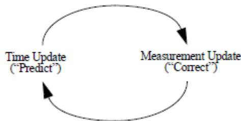
Figure 1. The ongoing discrete Kalman filter cycle.
