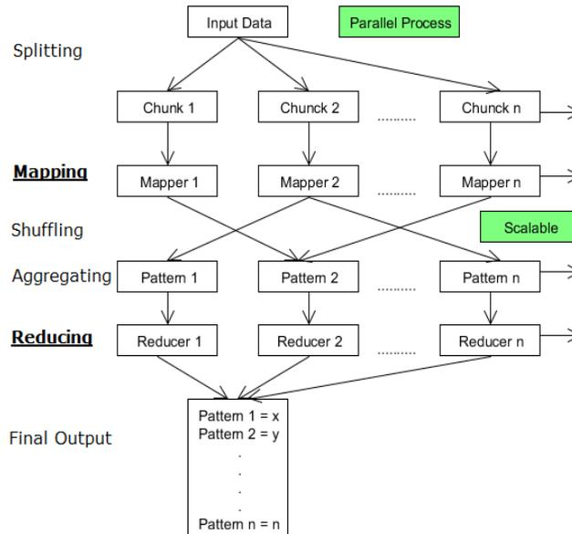
Fig. 5 Map Reduce Block Diagram [11]
