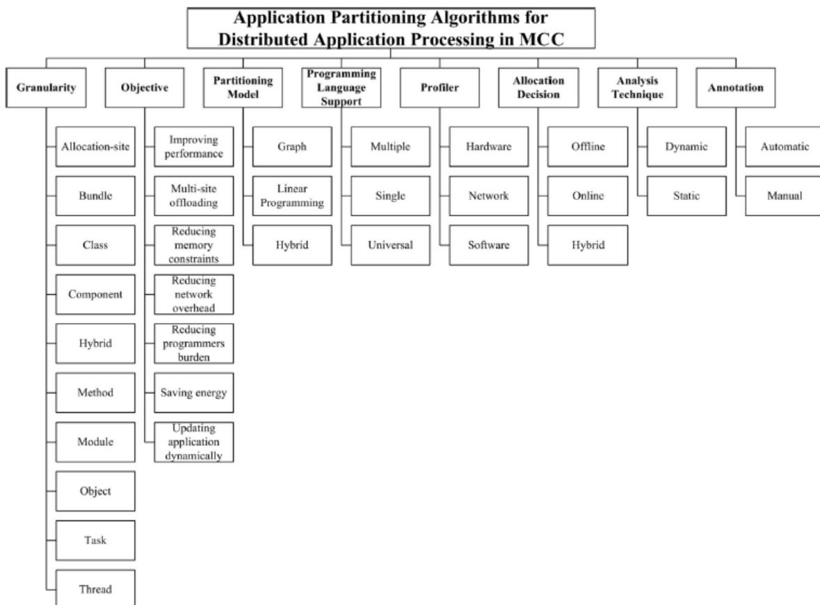
**Fig. 5. Application partitioning algorithms for distributed application processing in MCC**
