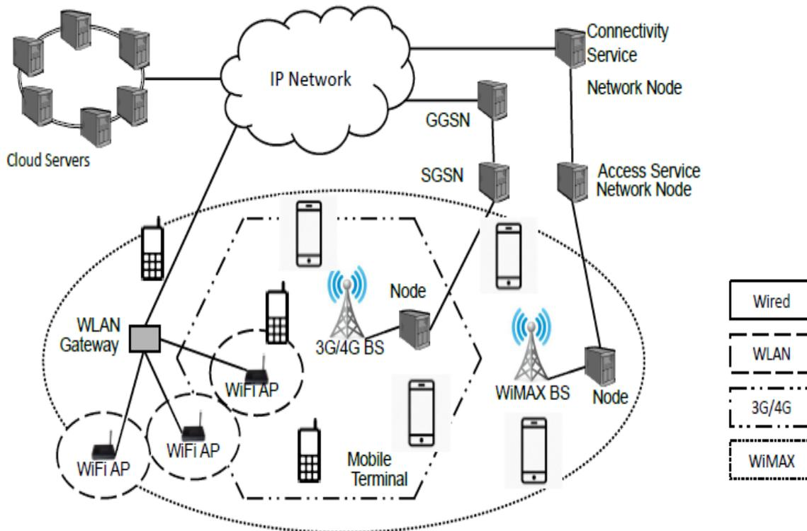
**Fig. 1. Mobile cloud computing uses everywhere mobile phones connect to cloud servers via various network interfaces such as WiFi, cellular network, and WiMax**
