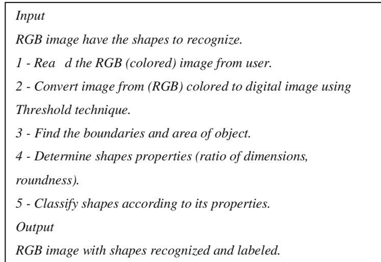
Fig 3.1 Procedure for Shape Detection
