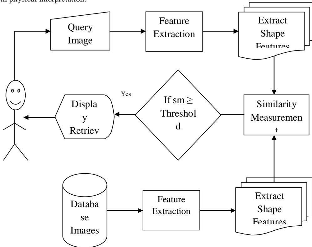
Fig 3.6 Diagram for Shape Based Image Retrieval
