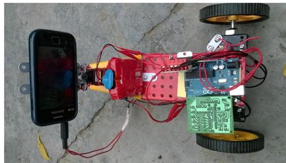
Fig 6 Car with phone attached
