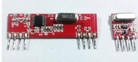
Fig 2 Receiver and transmitter modules
