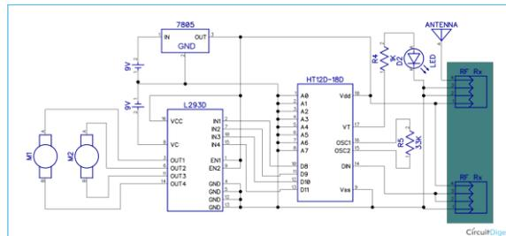
Fig 3 circuit diagram of car module
