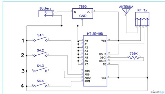
Fig 4 circuit diagram of control module
