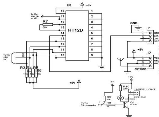
Fig 5 Circuit diagram
