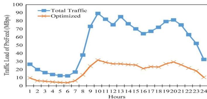
Figure 3: Traffic load without and with PreFeed.
